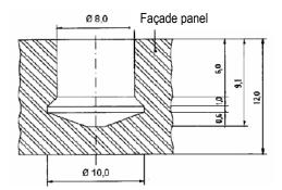
After the anchor has been inserted into the pre-drilled undercut hole (A + B), its sleeve is splayed into the desired position by insertion of the screw (C).
