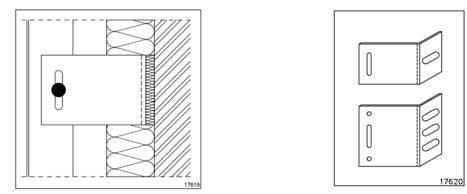
The distance between the brackets is determined by the load exerted (as a result of the wind load and force of gravity) and the strength properties of the aluminium sections (to be indicated by the supplier of the aluminium supporting structure). The calculation of the wind load has to be done according to the national applying standards (NBN B 03-002-1; NEN 6702:2001; NBN-EN 1991-1-4).
