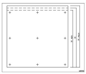
Each panel can cope with a vertical tolerance of -15 mm to +15 mm in the building. Cut-to-fit panels should be ordered with a height 15 mm greater than the desired height. The edge distance of the undercut holes from the top edge of the panel normally measures 100 mm, but can lie between 70 and 100 mm.
