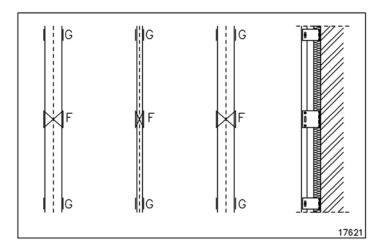
The fixed fastening points are located at the same height so that stress in the sheet is avoided.
