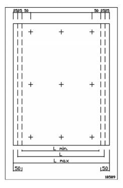
Each panel can cope with a horizontal tolerance of -50 mm to +50 mm in the building. Cut-to-fit panels should be ordered with a width 50 mm greater than the desired width. The distance of the undercut holes to the vertical panel edges normally measures 100 mm, but can lie between 50 en 100 mm.
