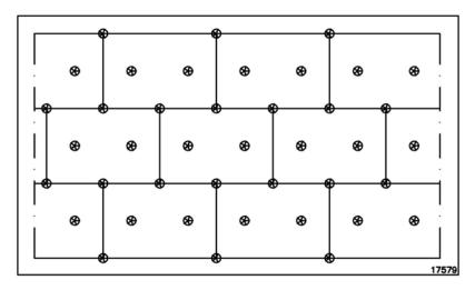
If the supporting profiles are fixed with brackets, the insulation is fastened after the fitting of the brackets and before the fitting of the supporting profiles. A slit is cut in the insulation at the bracket.
